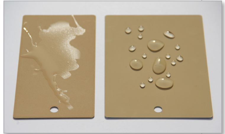
Panel with hydrophobic Chemical Agent Resistant Coating applied
