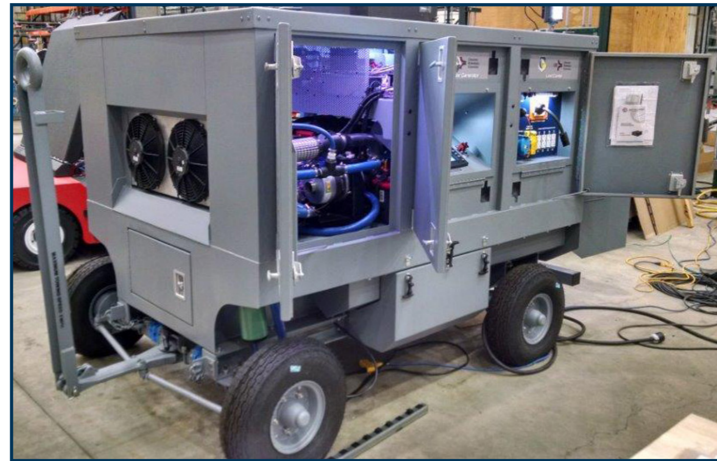
12kW Fuel Cell Power
