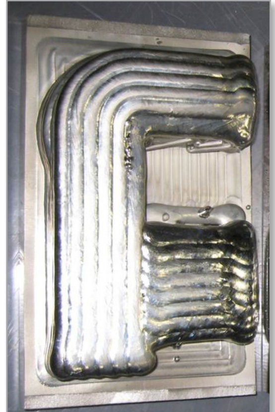
Development of effective NDI methods is critical to ensure implementation of EBDM components on the F-35. (Sciaky photo)
