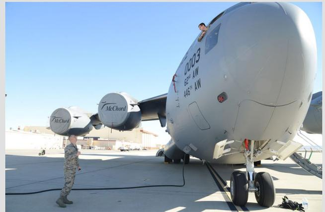
Staff Sgt. Steven Schrader (left) and Staff Sgt. Alex Rini, 412th Logistics Test Squadron, discuss the progress of the C-17 portion of the Hybrid Electric Flightline Cart Technology Pathfinder tests. The nearly zero noise of the HEF allows maintainers to converse without the use of the aircraft’s internal communication system. (U.S. Air Force photo by Christopher Ball)
