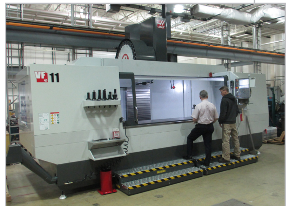
The hybrid directed energy deposition AM machine in a Haas VF 11 multi-axis machine tool.
