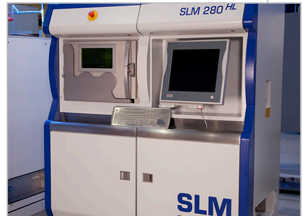
With the SLM 280 HL , we create metal parts using various materials including aluminum, titanium, stainless steel, cobalt-chromium, and others.
