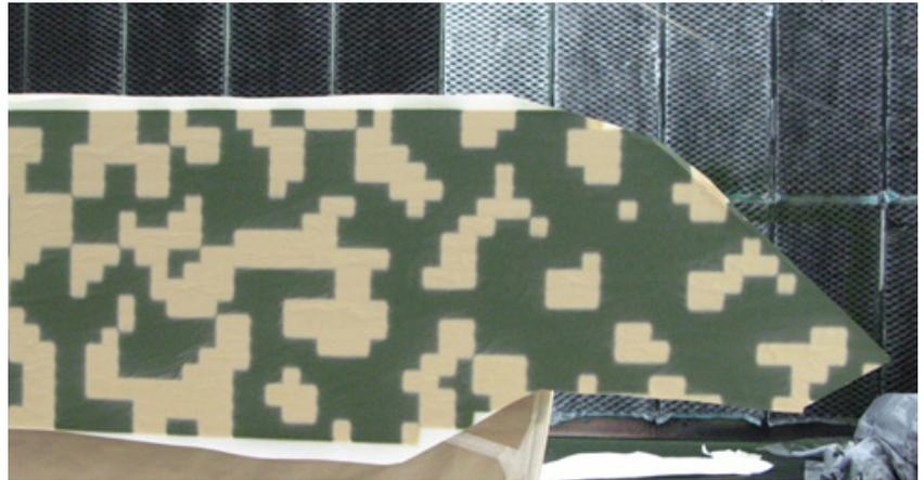
*From creation to integration, Concurrent Technologies Corporation Huntsville's Secure Design and Fabrication Facility offers clients unique, advanced services. Here, a weapon system receives digital camouflage using a proprietary robotic system and multiple spray guns.*
