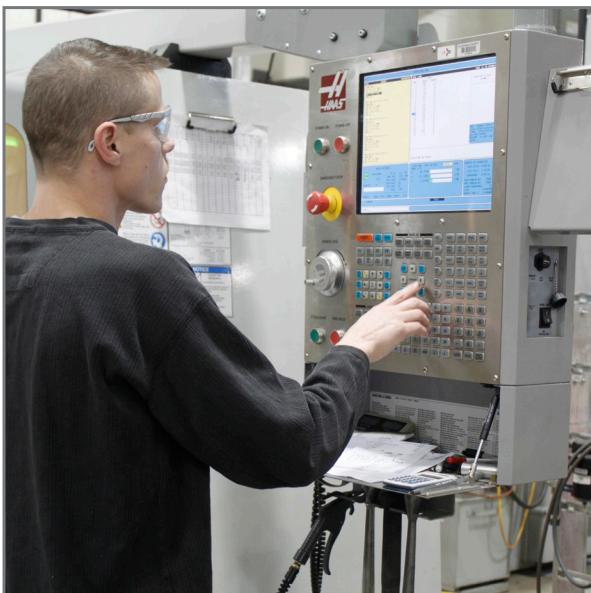
CTC utilizes offline Computer Numerical Control (CNC) programming to produce components. Benefits include minimum machine down time, consistent and accurate work pieces, and flexibility.
